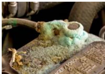
But often times, this can be easily treated by simply pouring a small amount of Cola or a DIY anti-corrosion paste (*one part water to three parts baking soda*) over the corroded areas.
