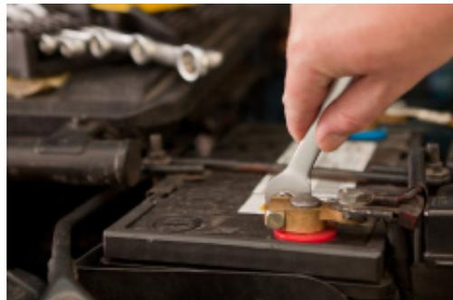
The same could happen if you have bad battery cables (or they're not connected properly). So check your cables and make sure they have a secure connection as well.
